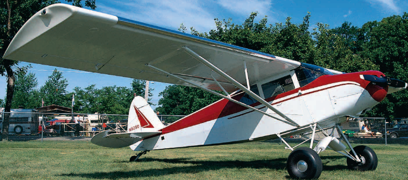
The slotted wing mod on the Ericksons' Pacer really works. "The airplane doesn't like to stall."
